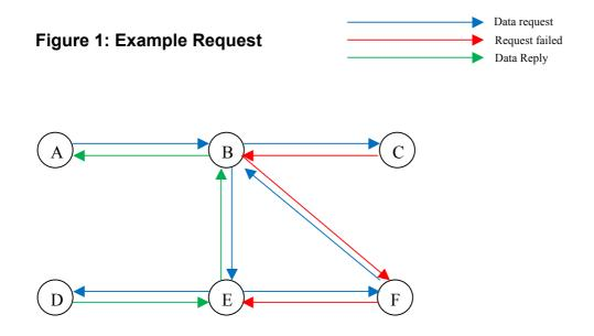
An example request. A requests data from B. B forwards request to C. C has no relevant contacts and so sends a failure message to B. B forwards the message to E. E forwards to F. F forwards to B. B recognises a loop has been made and sends a loop message to F. F has no more relevant contacts and sends a failure message to E. E forwards to D. D has the data and forwards it to E. E forwards the data to B. B Forwards the data to A.
